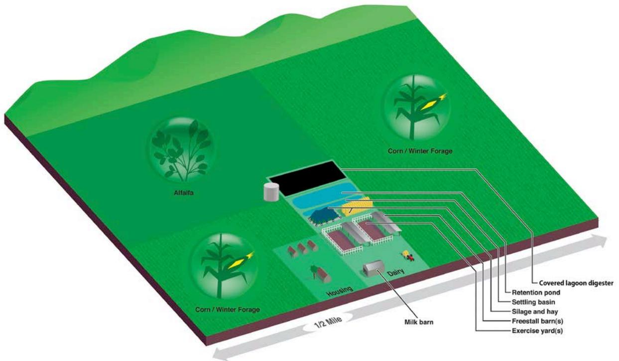
For purposes of analysis, each dairy is assumed to install a new Tier 1 (double-lined) lagoon with cover for digestion and biogas production. The distributed electricity generation model also assumed the installation of onsite electrical generation capacity sized to energy production potential and capable of meeting all local air quality permitting requirements. Caterpillar internal combustion engines with SCR NO<sub>x</sub> reduction were utilized.
