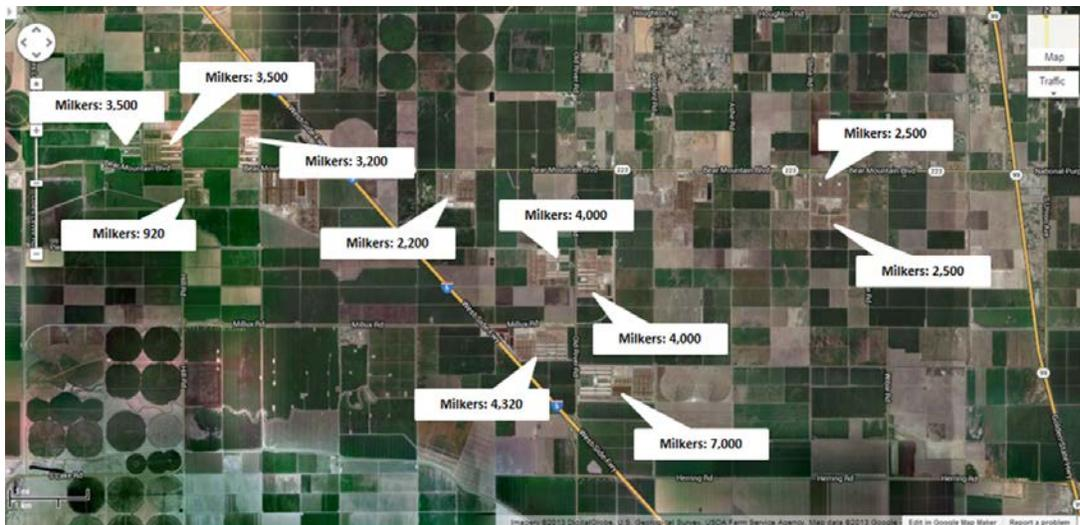
Approximately 7-10 miles of gas gathering pipeline would be needed to connect all dairies to a centralized hub.
