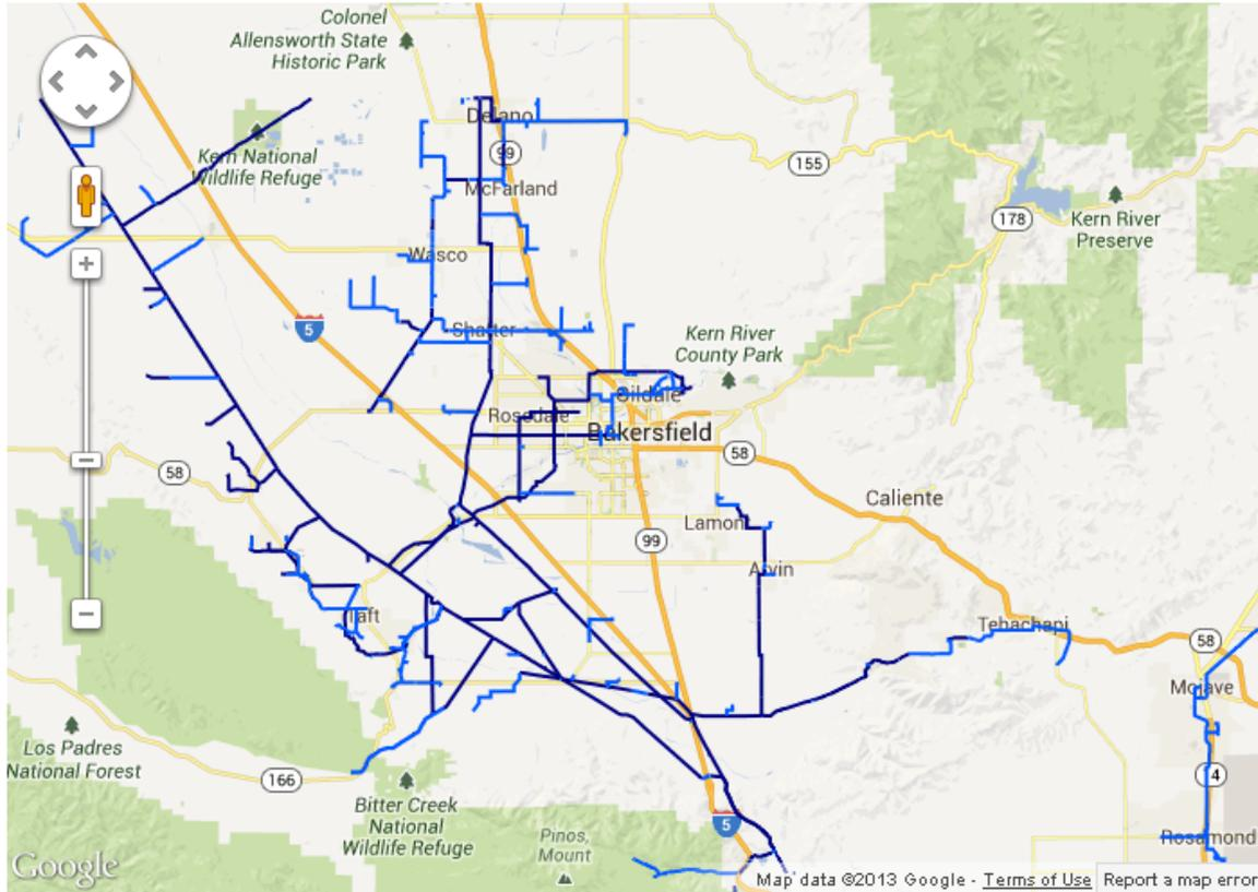
**Dark Blue** Transmission Lines: Generally large diameter pipelines that operate at pressures above 200 psi and transport gas from supply points to the gas distribution system.
